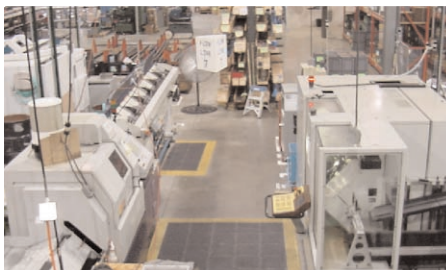
Bison motor shaft flow line. Ground and polished bar stock in background, lathe on left, hobbing machine on right.
